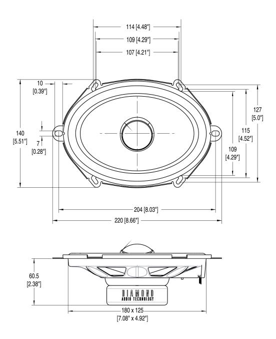
**M391i** General dimensions in millimeters and [inches]. Not to scale.
